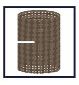
**Make** the basket frame using at least 12 big twigs or rafters inserted in a circle measuring 50 – 80 cm in diameter and 1.3 meters high. Acquire the smaller twigs around the frame.
