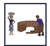
**Construct** the 1 meter wall structure from foundation by mixing anthill soil with water.
