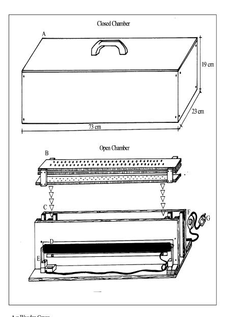
$\begin{array}{l} A = \text{Wooden Cover} \\ B = \text{Test Tube Rack} \\ C = \text{Lateral Walls} \\ D = \text{Lateral Window} \\ E = U.V. \text{Lamp-Mounting} \\ F = \text{Lamp Switch} \\ G = \text{Lamp Plug} \end{array}$
